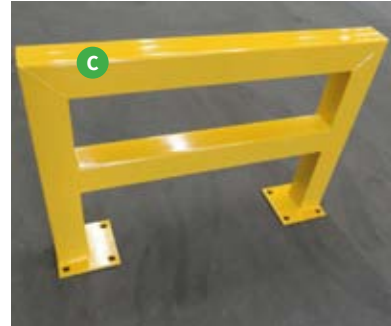
C SUBJECT: Bollards – 42" x 30" • HSS SQ. 4" x 4" x .125W construction • 8" x 8" x .5" base plate with four 1" holes for anchoring • Powder coated Unitran standard yellow
