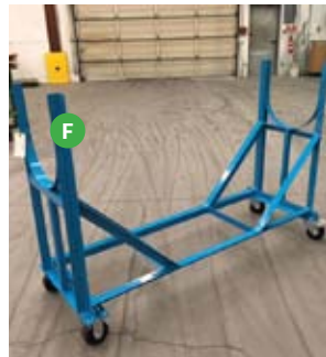
F • 26" x 72" x 48" AOH • 2" x 2" x .1875" angle iron construction • 2" x 10GA tube cradle with HHS SQ. 1.5" x 1.5" x .188W vertical support • 5" phenolic swivel caster with brake and rigid casters • Powder coat Finish • Capacity - 3000 lbs.
