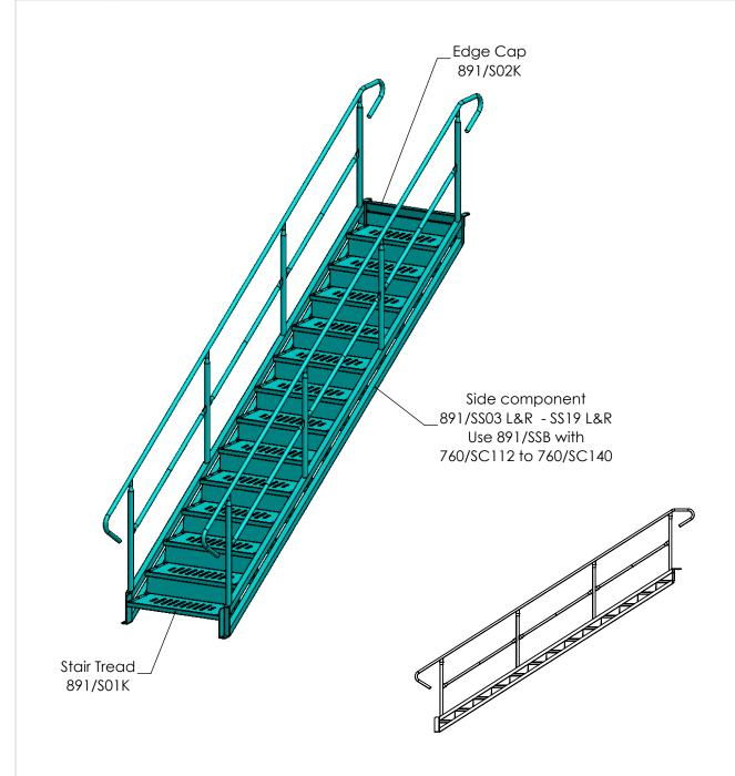
Use applicable fasteners and anchors
