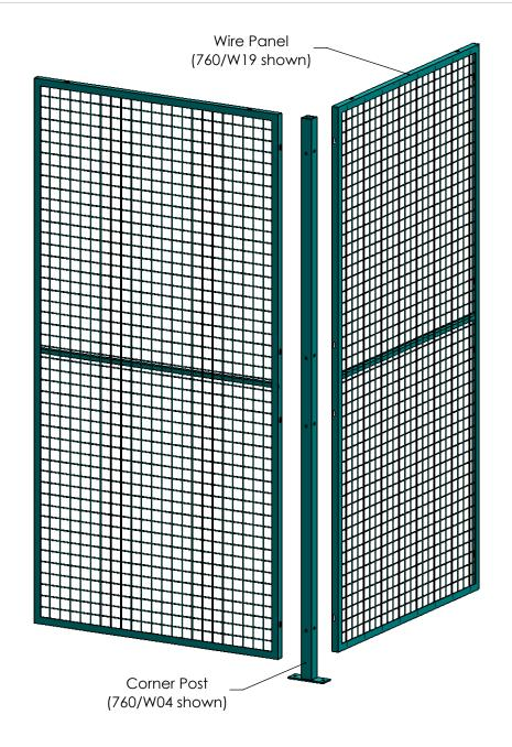
For anchoring post to floor use: 760/F03 (2 each) or 760/F031
